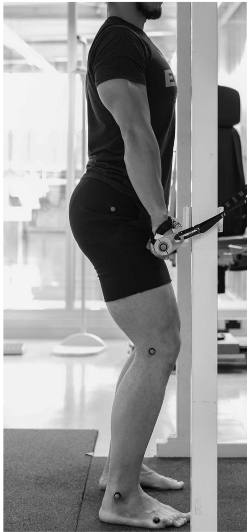
Figure 1. Isometric midhigh pull setup for a fixed-bar system. The bar is fixed using an inverted cable rack attachment with ratchet straps keeping it secured from above.
