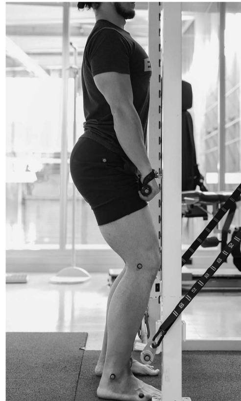
Figure 2. Isometric midhigh pull setup for a chain-based system. The bar is fixed just above the feet to simulate the attachment of the chain to the ground. This enables the force plate to measure the GRF at the same time the load cell measures the force through the chain.
